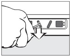
■ Use a screwdriver to push the emergency door latch downwards (see illustration). The drum door will open.
